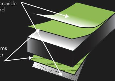
Black core made up from layers of kraft paper impregnated with phenolic thermosetting resins to give inner strength and durability
