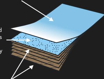
Layers of kraft paper impregnated with phenolic thermosetting resins to give inner strength and durability
